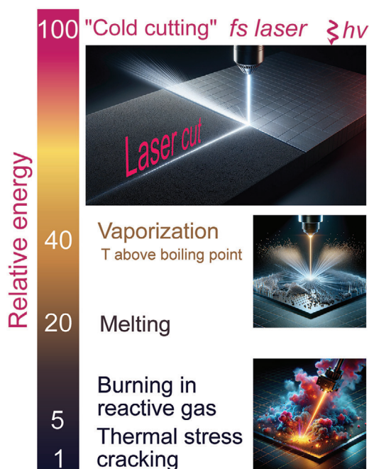
Figure 13. Progressive effects of increasing laser energy on a material's surface. At low energy, thermal stress and cracking occur, reaching burning in reactive gas, melting, and vaporization as energy levels rise. At the highest energy, "cold cutting" with a femtosecond laser is achieved, resulting in a precise and clean cut through the material.
